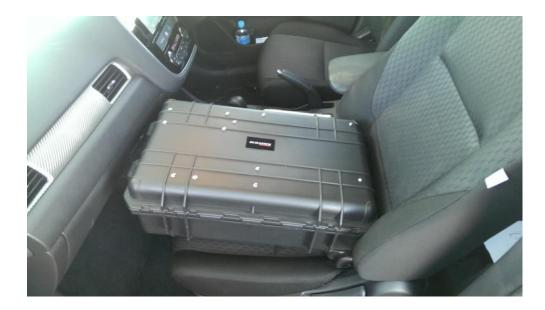
To activate the system, the case is opened, the power cord is plugged into the 'cigarette lighter' 12-volt power outlet and the inlet tube is clipped to the top of the window glass in the passenger door. The front passenger window is left slightly open to accommodate the air inlet tube. All of the equipment is hard wired to the power supply so that a single switch turns everything on or off.
